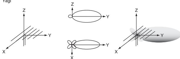
Figure 8: Antenna Radiation Patterns
