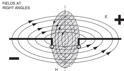
Figure 2: E and H Field Surrounding an Antenna
