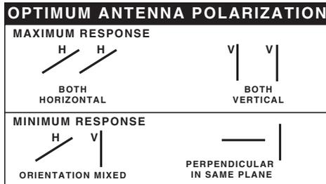
Figure 11: Antenna Polarization
