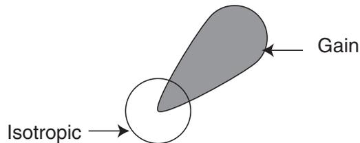
Figure 10: Antenna Gain
